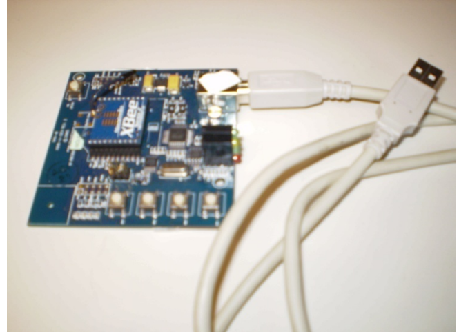
Figure 2. USB ZigBee enabled device with wire antenna
