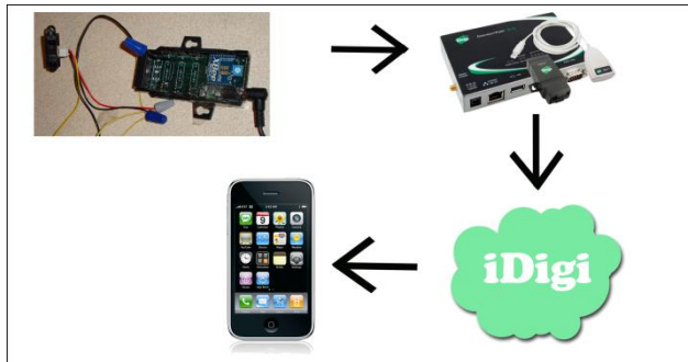
Figure 4. Flow of data from sensor to gateway to iDigi to iPhone
