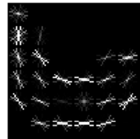
Figure 5. Histogram of oriented Gradients banana
